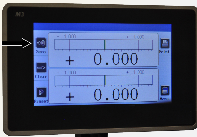
Fig. 50: Reset measuring probe
