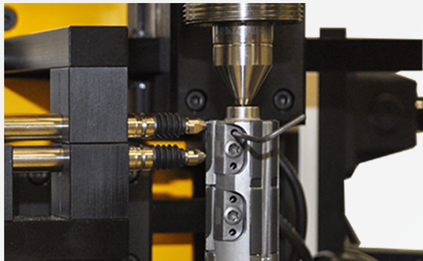
Fig. 54: Set upper radial adjusting screw
