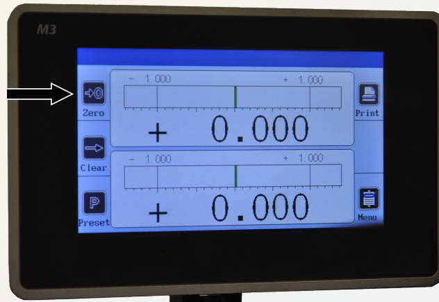
Fig. 48: Reset measuring sensor
